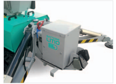
Lithium batteries compartment: protected and easily accessible for the charging cycle management.
