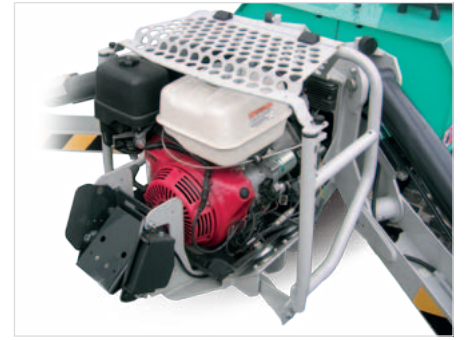
Rugged engine guard for improved protection.
