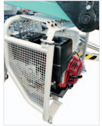
Strong protective engine structure for an increased impact protection.
